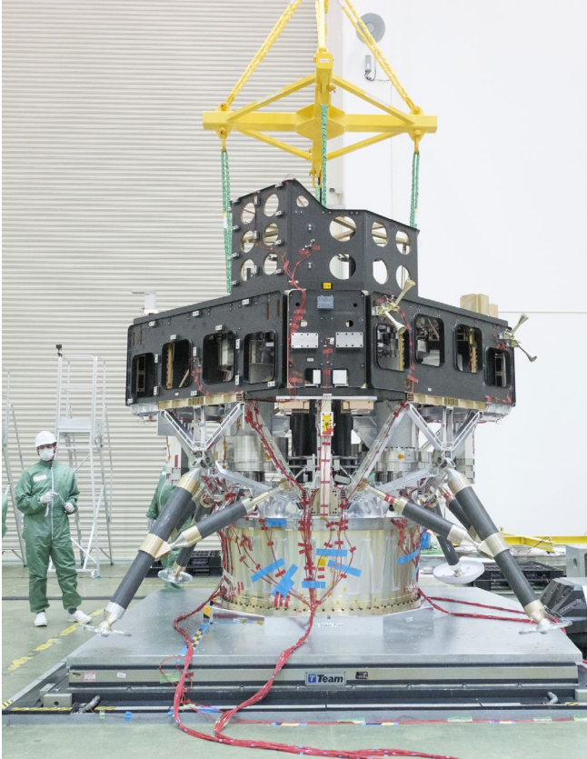
Photo taken during vibration testing of the ULTRA lander, currently under development with support from METI's SBIR program.
