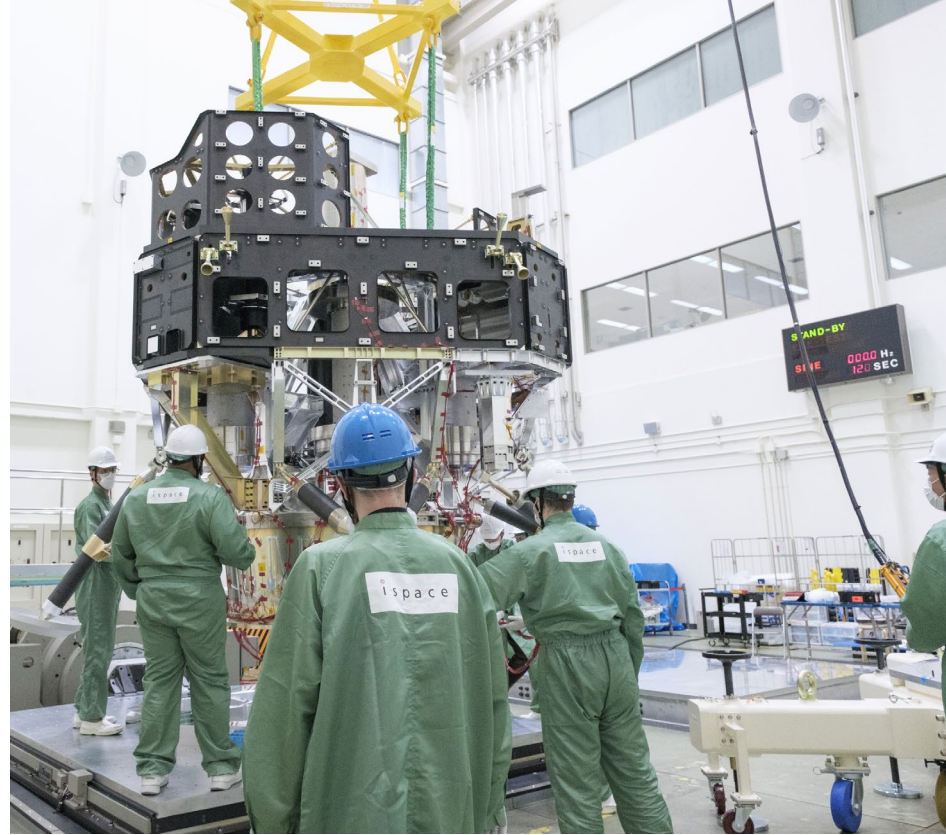
Photo taken during vibration testing of the ULTRA lander, currently under development with support from METI's SBIR program.
