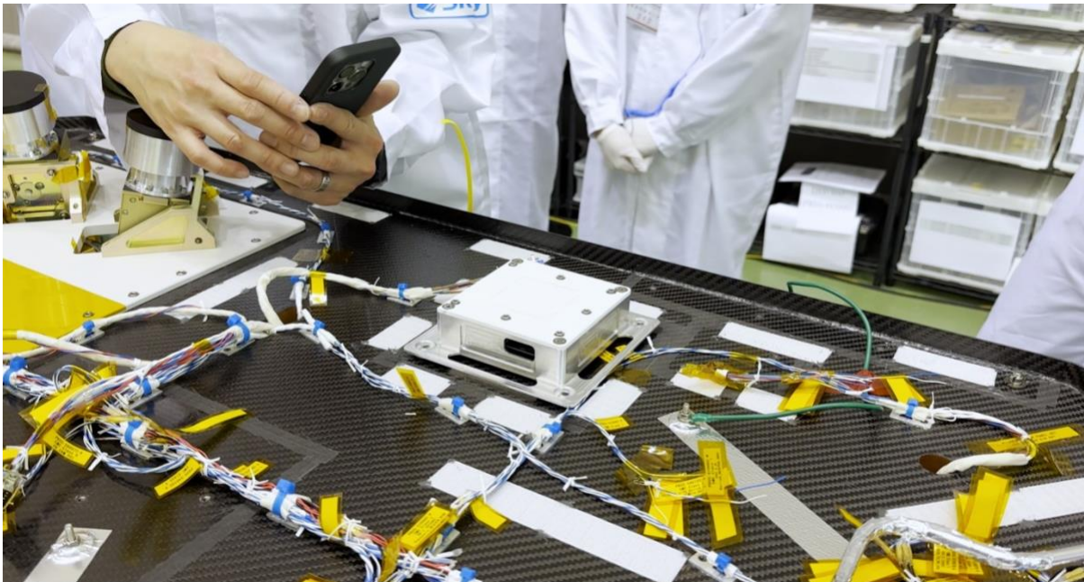
An image of the Deep Space Radiation Probe developed by the National Central University of Taiwan as it was being installed into ispace's RESILIENCE lunar lander.
