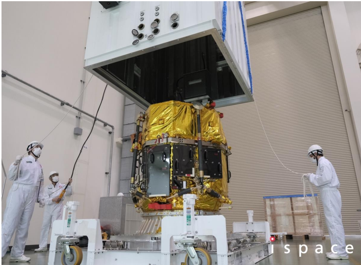
Photo: ispace engineers load the Mission 2 RESILIENCE lunar lander into a transport container in preparation for shipping to Florida.
