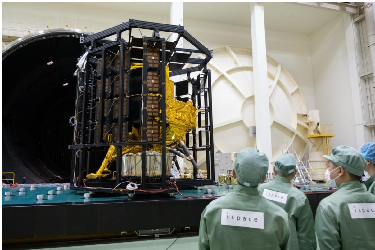
Engineers from ispace’s Assembly, Integration & Testing team oversee removal of the Series 3 Lunar Lander Structural Thermal Model from the Thermal Vacuum Testing chamber at a JAXA facility in Tsukuba, Japan.
