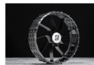
(Left Image) concept model of a tire developed by Bridgestone for lunar rovers
