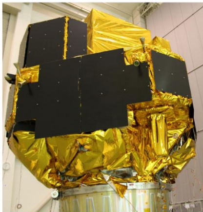
Photos of the structural thermal model of tentatively named Series 3 lander under development with METI's SBIR grant
