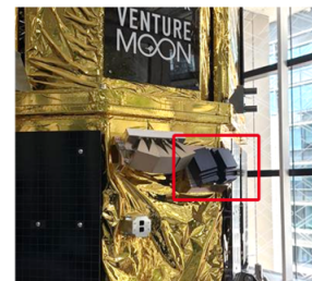
In the above photo, the red frame shows the LRF. It is installed on the side of the lander.
