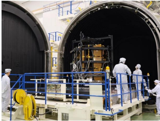
ispace engineers moving the RESILIENCE lunar lander into a testing chamber at a JAXA facility in Tsukuba, Japan
