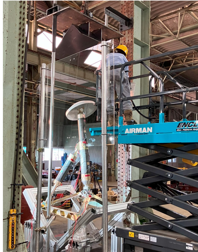
Drop weight testing of the structural thermal model of tentatively named Series 3 lander under development with METI's SBIR grant
