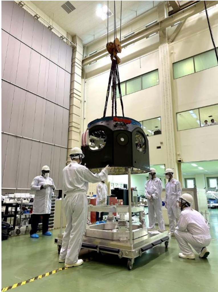
Left image : Conducting assembly operations of monocoque of the lander at the facility held by JAXA Top right image : Conducting taping operations inside monocoque for heat control at the facility in Germany Bottom right image: Installing wire harnesses at the facility held by JAXA
