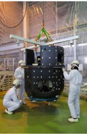
Photos of the structural thermal model of the HAKUTO-R M2 lunar lander being assembled at a Japan Airlines Facility in Narita Airport.
